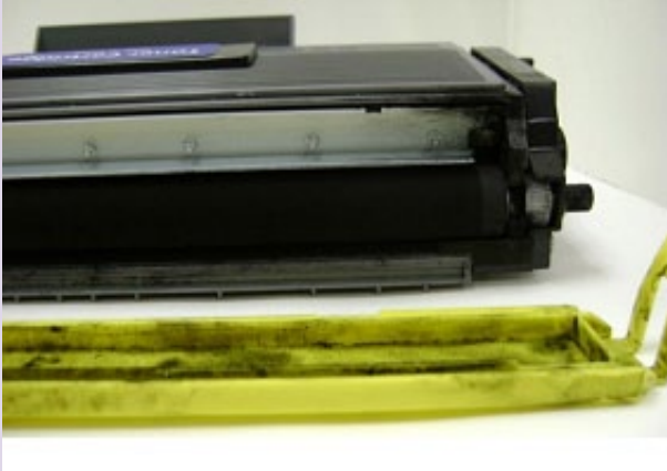
Example of toner leakage with a newly opened aftermarket cartridge.
