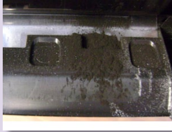
Example of toner leakage while printing with an aftermarket cartridge.
